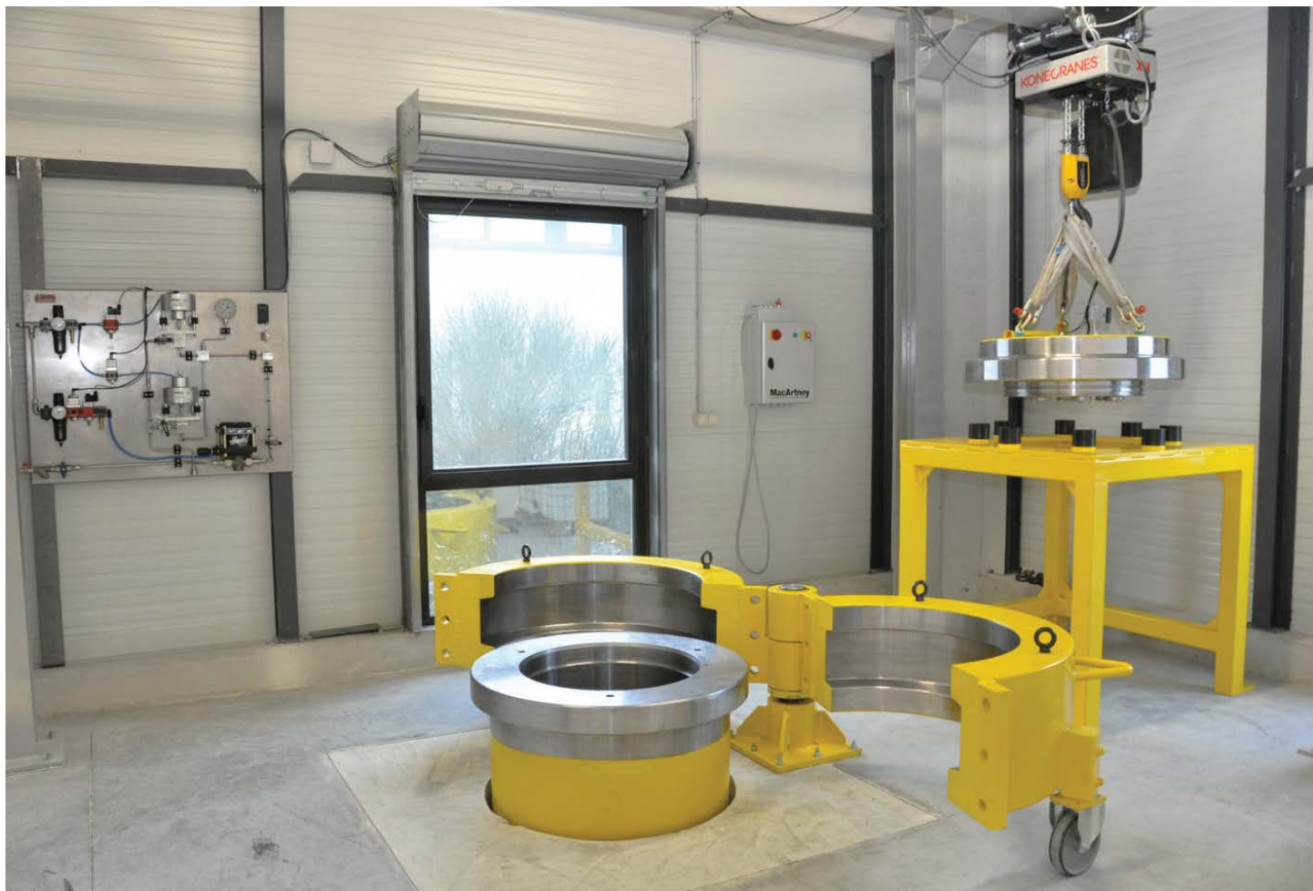
A MacArtney hydrostatic pressure vessel has been installed within a new test environment. (Source: MacArtney)
